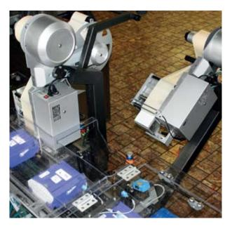
Via a specially designed swivelling arm, one system can be swung clear of the line for replenishement, while a second unit takes over the labeling of up to 60 cases per minute.
